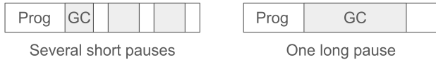
Figure 2. Cheng and Belloch [13] used a figure like this to illustrate the problem with using GC pauses as a measure of responsiveness and proposed the minimum mutator utilization (MMU) metric as a response. GC pause time continues to be widely (mis)used as a proxy for responsiveness more than twenty years later.
